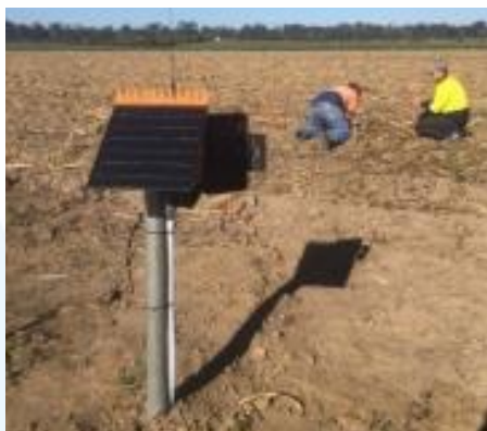
Solar powered probes send data by telemetry
